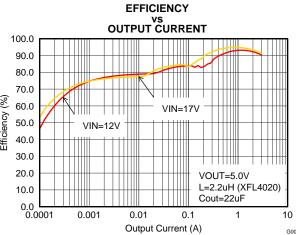
Figure 7. Efficiency with 2.5MHz, Vout=5V
