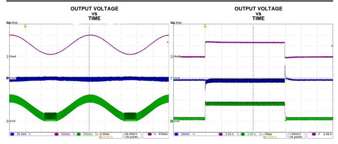
Figure 29. PWM-PSM-Transition (V $_{\rm IN}$ =12V, V $_{\rm OUT}$ =3.3V with  $50 {\rm mV/div})$
