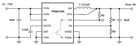
Figure 51. Discharge Vout through PG pin
