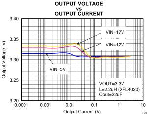
Figure 17. Output Voltage Accuracy (Load Regulation)
