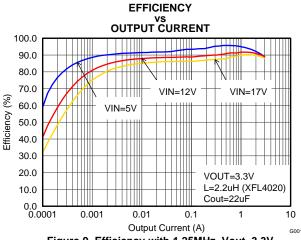
Figure 9. Efficiency with 1.25MHz, Vout=3.3V
