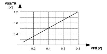
Figure 39. Voltage Tracking Relationship
