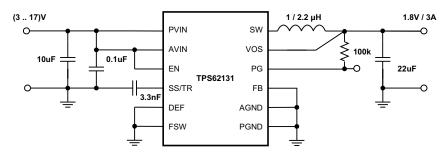
Figure 46. 1.8V/3A Power Supply
