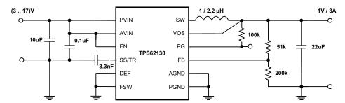
Figure 49. 1V/3A Power Supply
