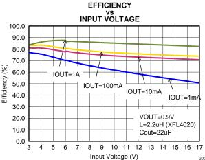
Figure 16. Efficiency with 1.25MHz, Vout=0.9V
