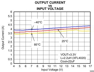
Figure 26. Maximum Output Current
