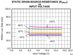
Figure 24. Low-Side Switch Resistance
