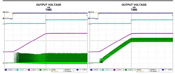
Figure 33. Startup into 100mA (VIN=12V, VOUT=3.3V)
