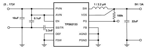
Figure 43. 5V/3A Power Supply
