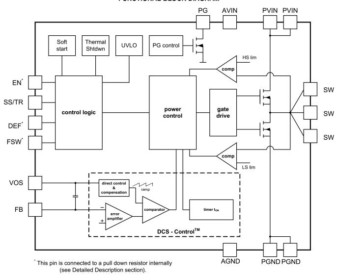
Figure 2. TPS62130 (adjustable output voltage)
