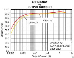
Figure 5. Efficiency with 1.25MHz, Vout=5V
