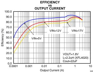
Figure 13. Efficiency with 1.25MHz, Vout=1.8V
