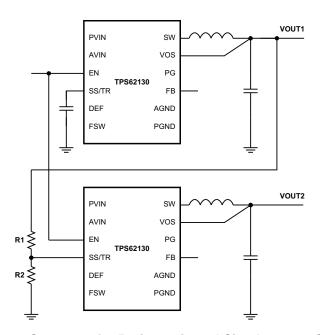
Figure 40. Sequence for Ratiometric and Simultaneous Startup
