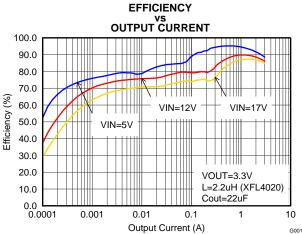
Figure 11. Efficiency with 2.5MHz, Vout=3.3V
