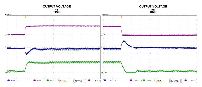
Figure 31. Load Transient Response of Figure 30, rising edge
