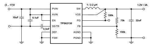
Figure 48. 1.2V/3A Power Supply
