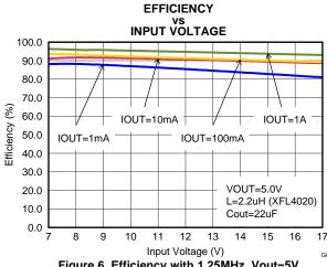
Figure 6. Efficiency with 1.25MHz, Vout=5V
