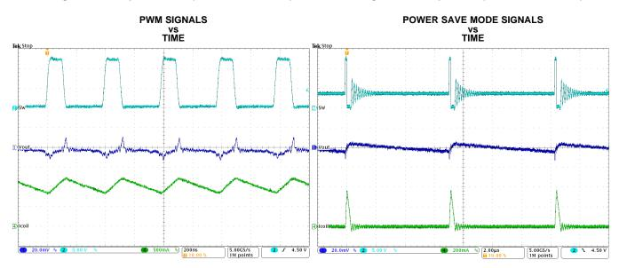
Figure 35. Typical Operation in PWM Mode (I<sub>OUT</sub>=1A)
