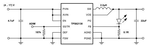
Figure 42. Single Power LED Supply
