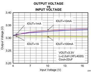
Figure 18. Output Voltage Accuracy (Line Regulation)
