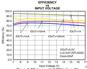
Figure 8. Efficiency with 2.5MHz, Vout=5V
