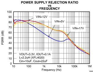
Figure 28. Power Supply Rejection Ratio, f<sub>SW</sub>=2.5MHz
