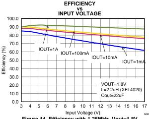
Figure 14. Efficiency with 1.25MHz, Vout=1.8V
