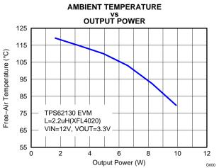
Figure 38. Maximum Ambient Temperature (f<sub>SW</sub>=2.5MHz)
