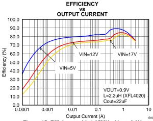
Figure 15. Efficiency with 1.25MHz, Vout=0.9V
