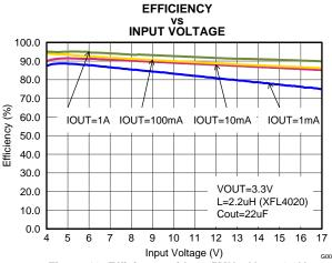
Figure 10. Efficiency with 1.25MHz, Vout=3.3V
