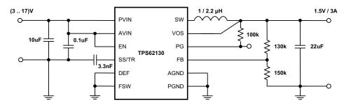
Figure 47. 1.5V/3A Power Supply
