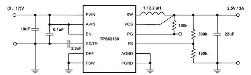
Figure 45. 2.5V/3A Power Supply
