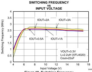
Figure 19. Switching Frequency
