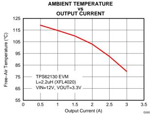
Figure 37. Maximum Ambient Temperature (f<sub>SW</sub>=2.5MHz)
