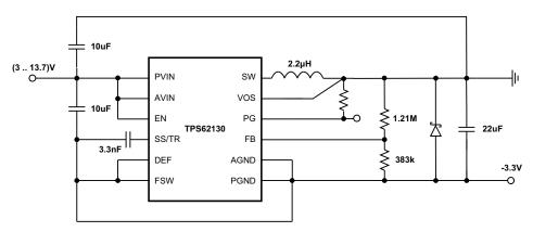
Figure 50. -3.3V Inverting Power Supply
