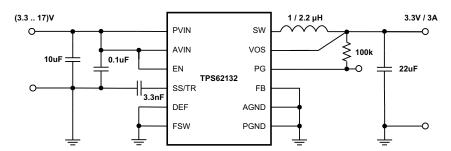
Figure 44. 3.3V/3A Power Supply
